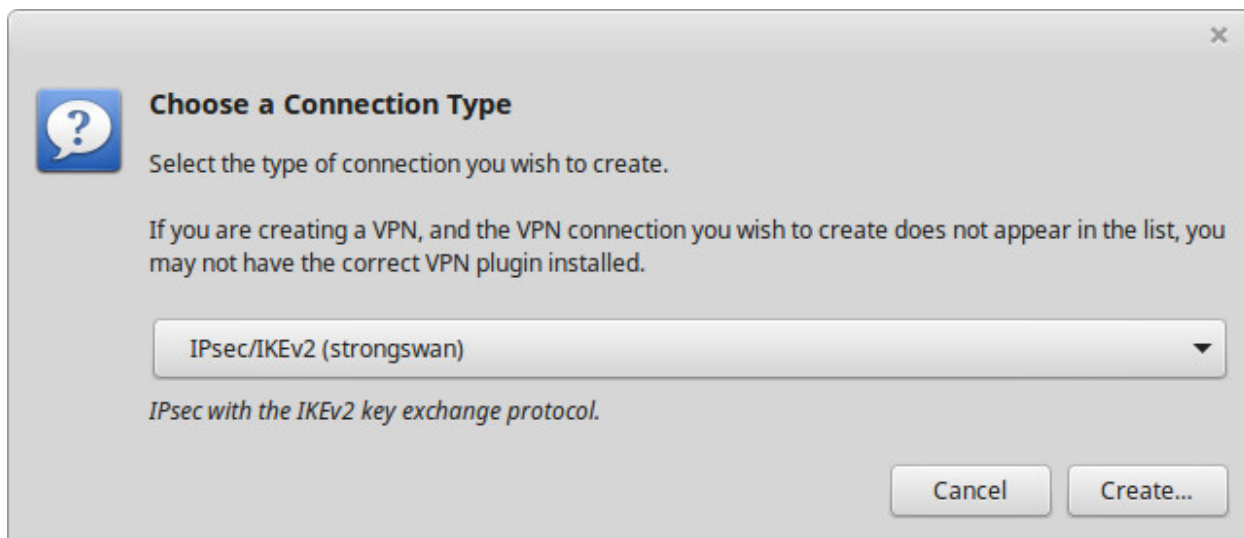
Fig. 33: Adding an IKEv2 VPN on Ubuntu
